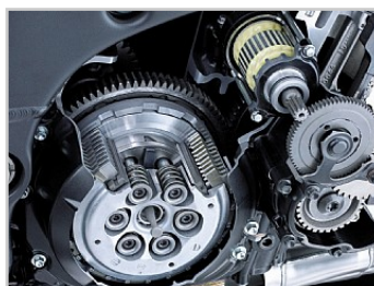
Adjustable back-torque limiting clutch
